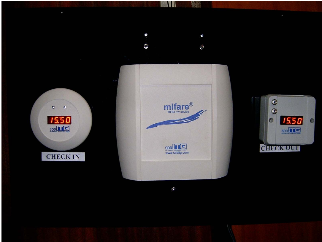
Fig.1 Terminal ITGsr-0x with two external antennae ITGant-07 (left: commercial housing, right: waterproof housing)
